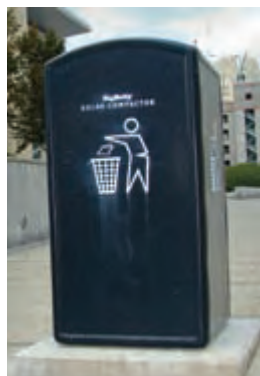
Big Belly solar-powered trash and recycling compactor.
